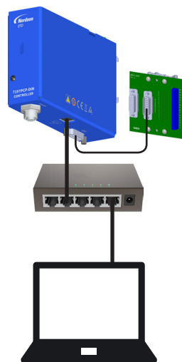
7197PCP-DIN Controller allows Internet-based control of the pumps
